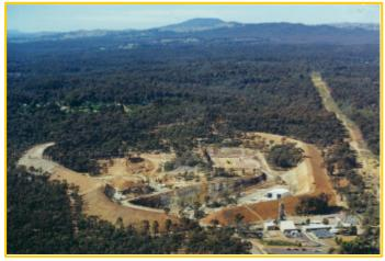
1999 – Development and progress. To minimise the impact on local residents an earth bund was constructed to attenuate noise.
